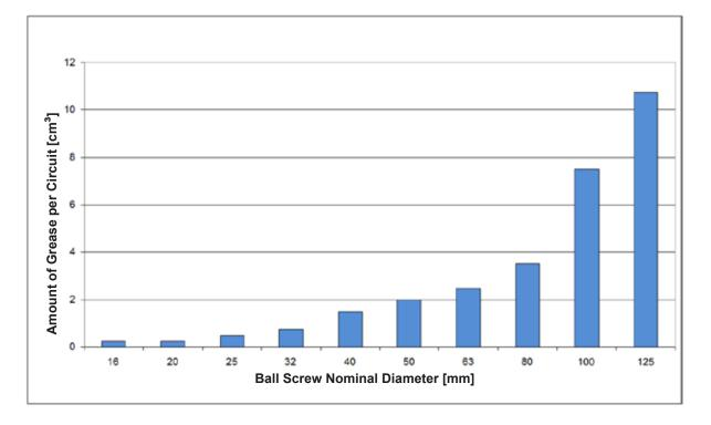
As a rule of thumb, replenish grease at least every 600-800 hours. However, because conditions vary so widely, you should confirm this interval by inspection and readjust if needed. For extreme conditions, consult a lubrication expert or ball screw manufacturer.
