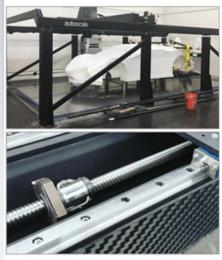
Autoscale's CNC technology (inset), which cuts objects up to 5 meters long, benefits from Thomson linear components, including precision ball screws and a profile rail that proved to be the only one long enough to meet their system requirements.
