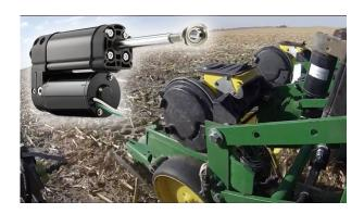
A prime example of this conversion was covered in a recent *Fluid Power World* article, which details Graham Electric Planter's electro-hydraulic actuator solution for optimizing seed depth control for multi-row agricultural planters. The Thomson H-Track actuator was at the core of Graham's development, delivering the required durability and communications capabilities.
