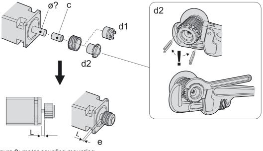
Figure 2: motor coupling mounting
