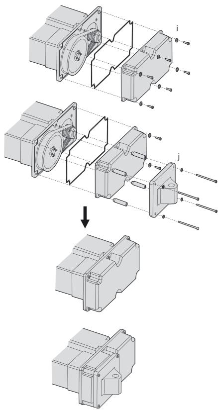
Figure 5: mounting of the cover
