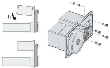
Figure 4: mounting of the belt
