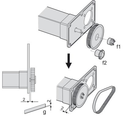
Figure 3: coupling to the unit
